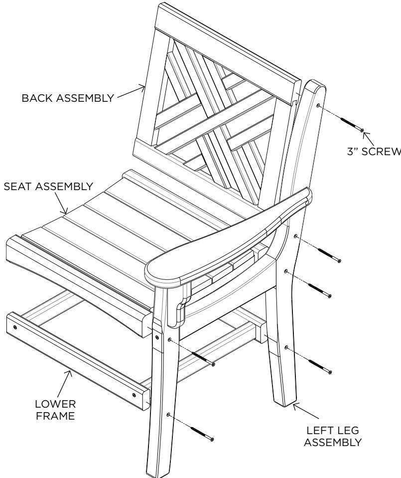
**STEP 2.** Use (6) 3" screws to attach the Right Leg Assembly to the Seat Assembly, Lower Frame, and Back Assembly.
